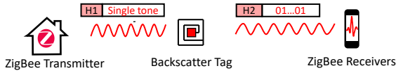
Fig. 2. System overview. The ZigBee transmitter provides RF carriers for signal excitation. The backscatter tag takes FPS to modulate ZigBee single-tone. Since RF carriers are dedicated resources for backscatter communication, the tag also translates the non-single-tone header (H1) into another (H2) to improve carrier utilization.
